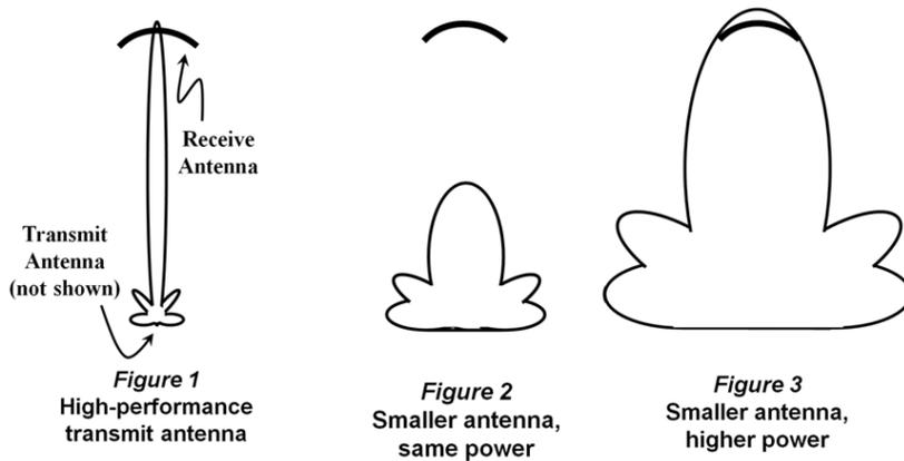
A smaller antenna spreads the signal in a broader pattern, with more leakage to the sides and back. Figure 2 shows a hypothetical smaller antenna, driven by a transmitter having the same power as in Figure 1.
